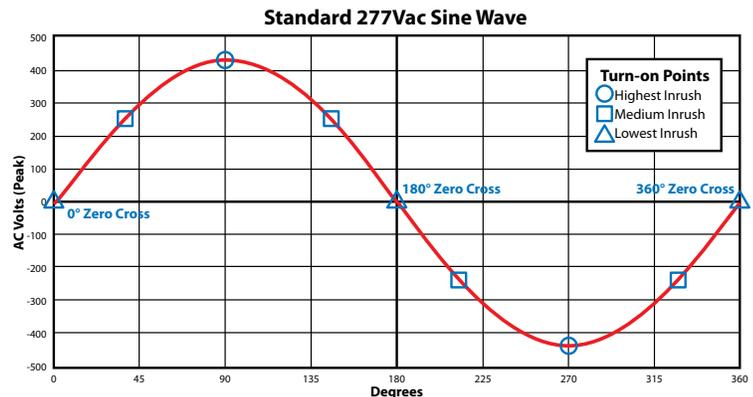
The inrush current spike itself has a magnitude and a width. It's normally characterized for its peak and time width (the time at which 10% magnitude occurs). It's also measured at some source impedance, the highest nominal AC line voltage of specified driver operation, full load, a nominal 25°C temperature, and a time at which it has not been recently switched on. The source impedance is a standard value given in NEMA 410.
